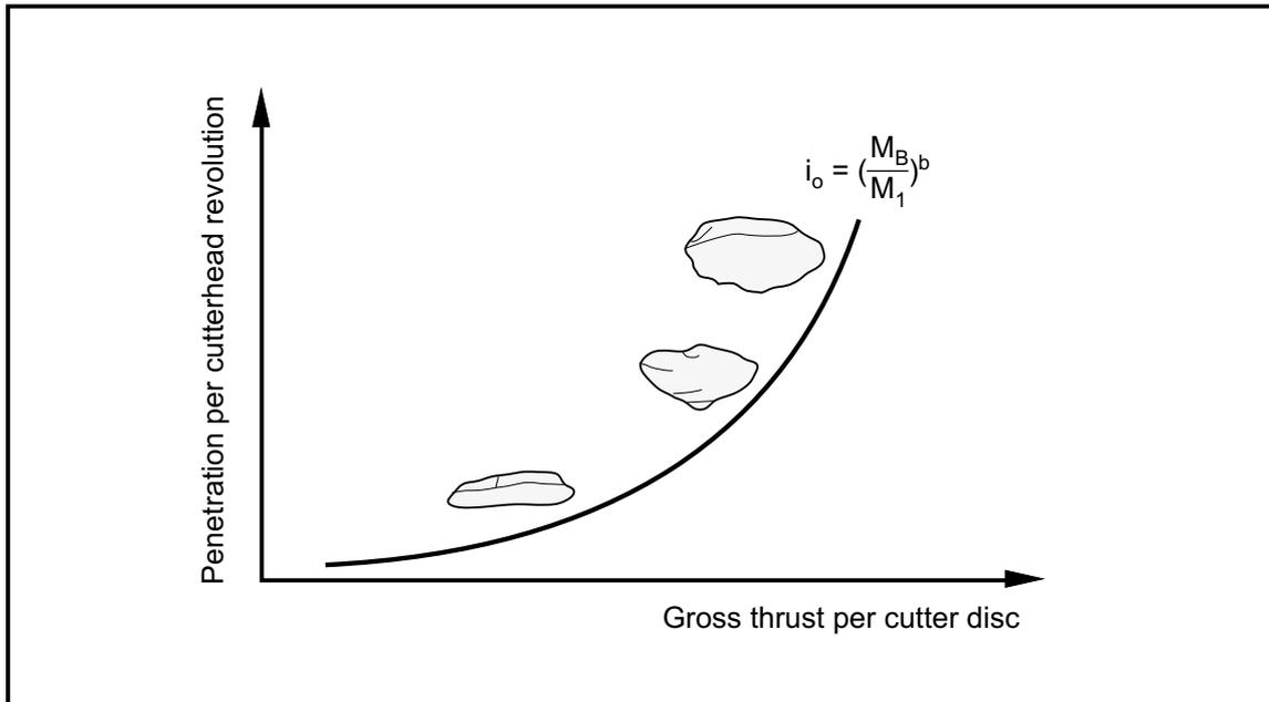
**Figure 3.1** General progress of a penetration test curve.
