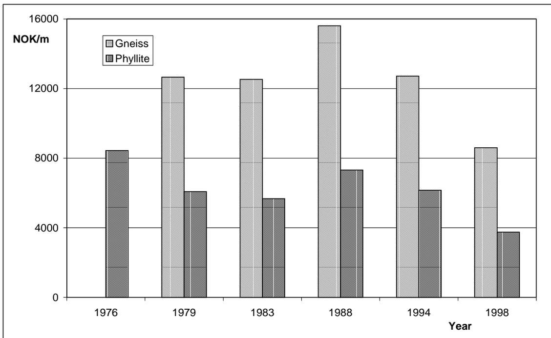
**Figure 3.4** Predicted excavation costs for a 3.5 m diameter TBM with 394 mm cutters. Price level of January 1999 [18].
