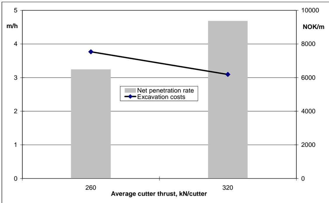
**Figure 2.2** *Influence of cutter thrust on net penetration rate and excavation costs for a 5 m diameter and 5000 m long tunnel in rock with  $DRI = 50$ , degree of fracturing = St I and  $\alpha = 30^\circ$  [7], [8].*
