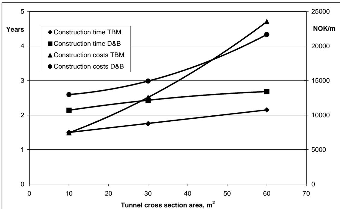
**Figure 2.3** Total construction time and total construction costs (1999 price level) for TBM and drill and blast tunnelling. Tunnel length 6 km. Rock conditions as in Figure 2.2 [18].
