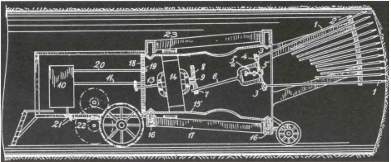
**Figure 2.1** *The patented tunnel boring device by Mr. I. Bøhn.*
