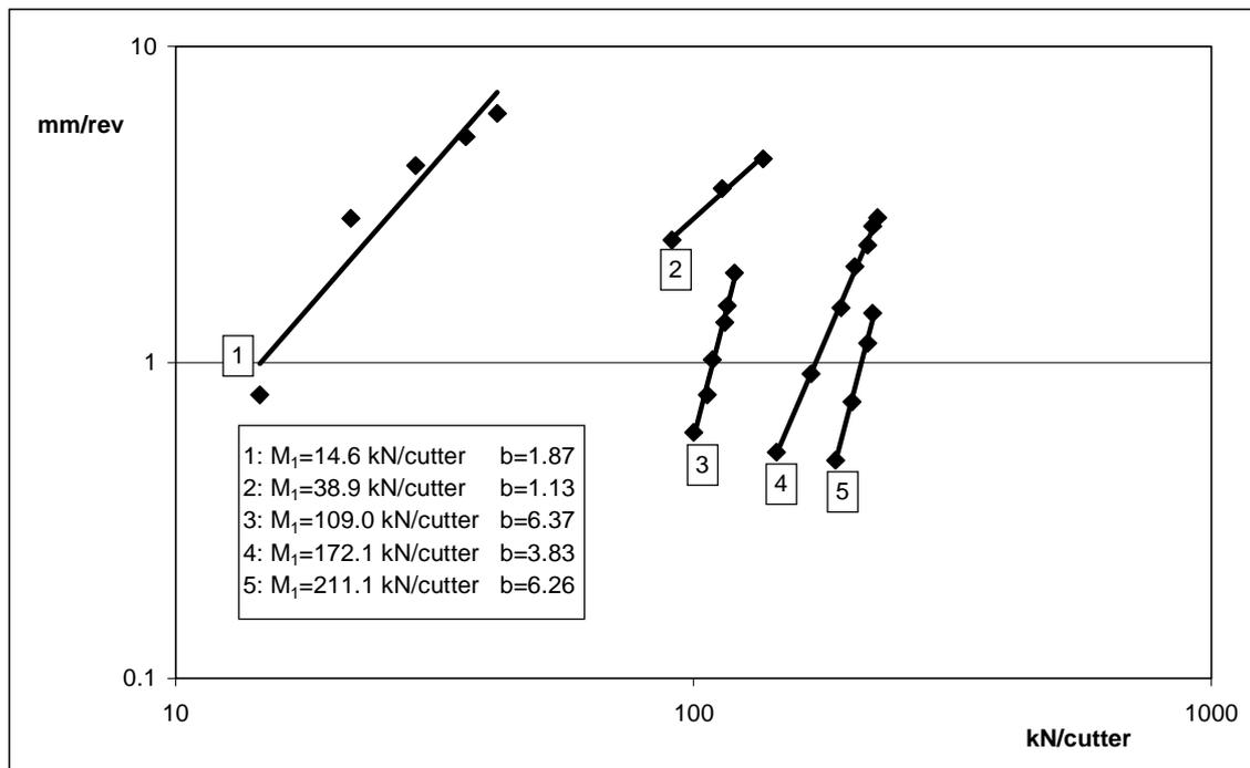
**Figure 3.2** Plot of some penetration tests.
